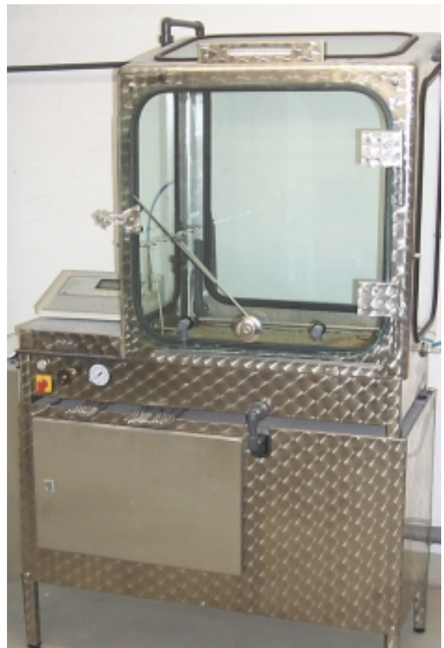
Fig. 3 Apparatus for accelerated artificial aging. (SO 2 )
