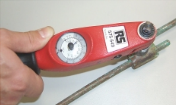
Fig. 4 Measurement of loosening torque
