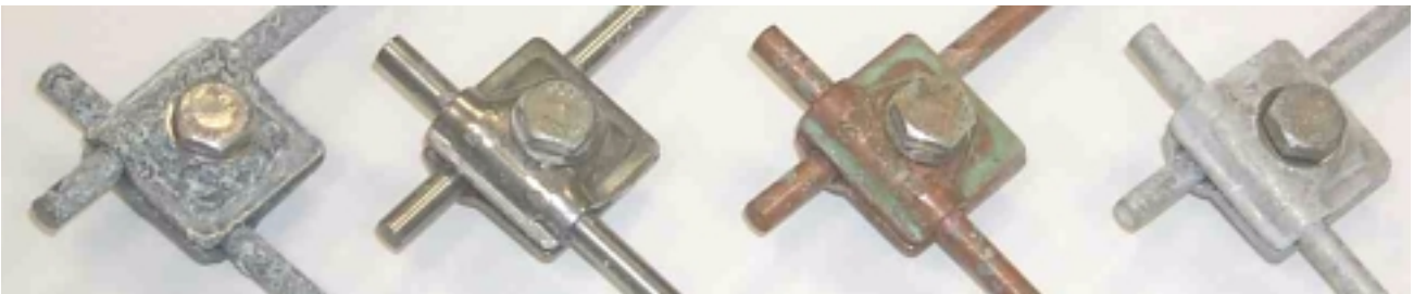
Fig.6 Arrangements after chemical treatment (Salt mist). All Bolts are made from stainless steel. Conductor and clamp, from left to right: hot dipped galvanized steel; stainless steel; copper, Aluminium.
