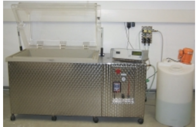
Fig.2 Apparatus for accelerated artificial aging.
