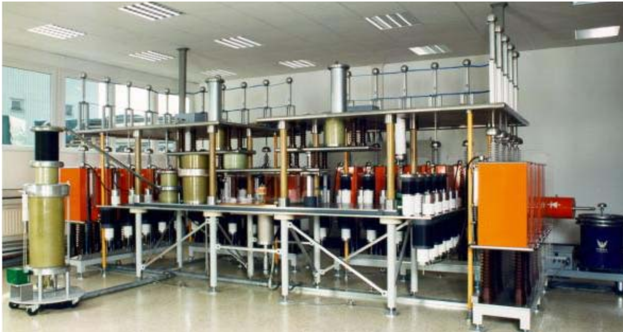
Fig 4 Crow bar generator for 200 kA /4/.
