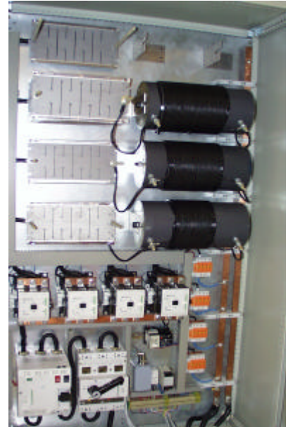
Fig. 2: Installation for the generation of follow currents with power frequency 50 Hz. Left: 10kV/250V Transformer. Right: Cabinet containing several switching devices and the additional coils and resistors for the shaping of the follow currents according to the standards.
