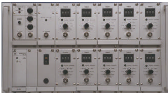
Fig.7 Digital multi channel time control unit. Resolution: 100ns. Optical outputs with laser impulse light.
