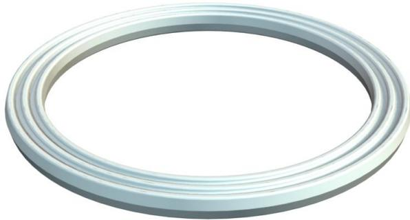
Connection thread sealing ring, suitable for all plastic cable glands, with metric thread according to DIN EN 60423 or ISO 68. The internal diameters of the sealing rings are designed in such a way that they can be pre-mounted in a captive manner.
