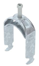
Clamp clip with hammerhead foot, metal pressure trough with rounded edges to protect the cable. For vertical and horizontal mounting of 1 single cable on a C-profile rail. For a slot width of 16–17 mm. With 1-start screw thread on pressure trough, universal hexagonal screw head WAF10, with slot and cross recess. Suitable for mounting indoors and outdoors. We recommend the use of a counter-trough.
