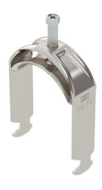
Clamp clip with hammerhead foot, metal pressure trough with rounded edges to protect the cable. For vertical and horizontal mounting of 1 single cable on a C-profile rail. For a slot width of 16–17 mm. With 1-start screw thread on pressure trough, universal hexagonal screw head WAF10, with slot and cross recess. Suitable for mounting indoors and outdoors. We recommend the use of a countertrough.
