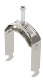
Clamp clip with hammerhead foot, metal pressure trough with rounded edges to protect the cable. For vertical and horizontal mounting of 1 single cable on a C-profile rail. For a slot width of 16–17 mm. With 1-start screw thread on pressure trough, universal hexagonal screw head WAF10, with slot and cross recess. Suitable for mounting indoors and outdoors. We recommend the use of a countertrough.
