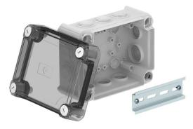
Junction box for the connection of cables and lines indoors and in protected outdoor areas. Rectangular design with plug-in seals to the sides and knock-out entries in the bottom. Suitable for wall and ceiling mounting and on mounting panels. With the option to fasten inside and to mount via the corner domes. High, transparent cover with quick lock, sealable. Made from halogen-free and UV-resistant materials.
