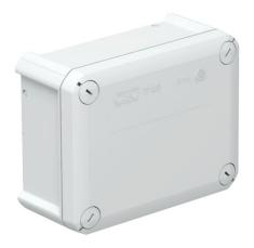
Junction box for the connection of cables and lines indoors and in protected outdoor areas. Rectangular design without entries. Suitable for wall and ceiling mounting and on mounting panels. With the option to fasten inside and to mount via the corner domes. Cover with quick lock, sealable. Made from halogen-free and UV-resistant materials.
