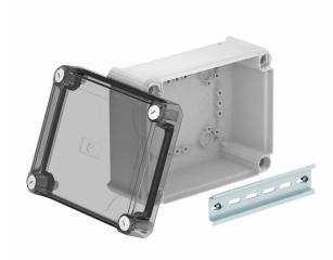
Closed junction box for the connection of cables and lines indoors and in protected outdoor areas. Rectangular design without entries. Suitable for wall and ceiling mounting and on mounting panels. With the option to fasten inside and to mount via the corner domes. High, transparent cover with quick lock, sealable. Made from halogen-free and UV-stabilized materials.
