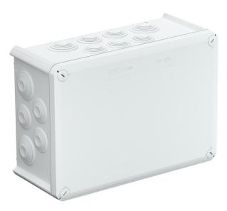
Junction box for the connection of cables and lines indoors and in protected outdoor areas. Rectangular design with plug-in seals to the sides and knock-out entries in the bottom. Suitable for wall and ceiling mounting and on mounting panels. With the option to fasten inside and to mount via the corner domes. Cover with quick lock, sealable. Made from halogen-free and UV-resistant materials.
