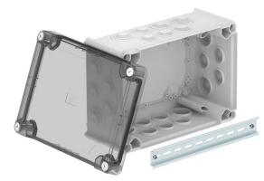
Junction box for the connection of cables indoors and in protected outdoor areas. Rectangular design with plug-in seals. Suitable for wall and ceiling mounting, on mounting panels and threads in the floor. With the option of fastening inside and to mount via the corner domes. High, transparent cover with quick lock, sealable. Made from halogen-free, UV-resistant materials.
