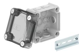
Junction box for the connection of cables indoors and in protected outdoor areas. Square design with plug-in seals to the sides and knock-out entries in the bottom. Suitable for wall and ceiling mounting and on mounting panels. With the option of fastening inside and to mount via the corner domes. High, transparent cover with quick lock, sealable. Made from halogen-free and UV-resistant materials.
