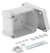
Junction box with hat profile rail for the connection of cables in indoor and outdoor areas. Rectangular design without entries. Suitable for wall and ceiling mounting with the option to fasten outside, inside or to mount via the corner domes. Particularly impact resistant with IK09. Cover with quick lock, sealable. Made from halogen-free and UV-resistant materials.
