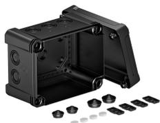
Junction box for the connection of cables and lines indoors and in outdoor areas. Rectangular design with knock-out entries. Suitable for wall and ceiling mounting with the option to fasten outside, inside or to mount via the corner domes. Particularly impact resistant with IK09. Cover with quick lock, sealable. Made from halogen-free and UV-resistant materials.
