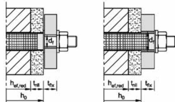
For through-setting installation, the annular gap between the anchor rod and the fixture must be filled with mortar.
