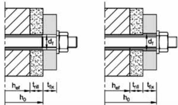
**Threaded rod M8 – M16 / Internally threaded anchor rod IG-M6 – IG-M10 with sleeve**
