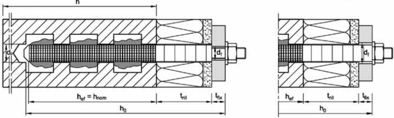
**Injection System VMU plus for masonry**
