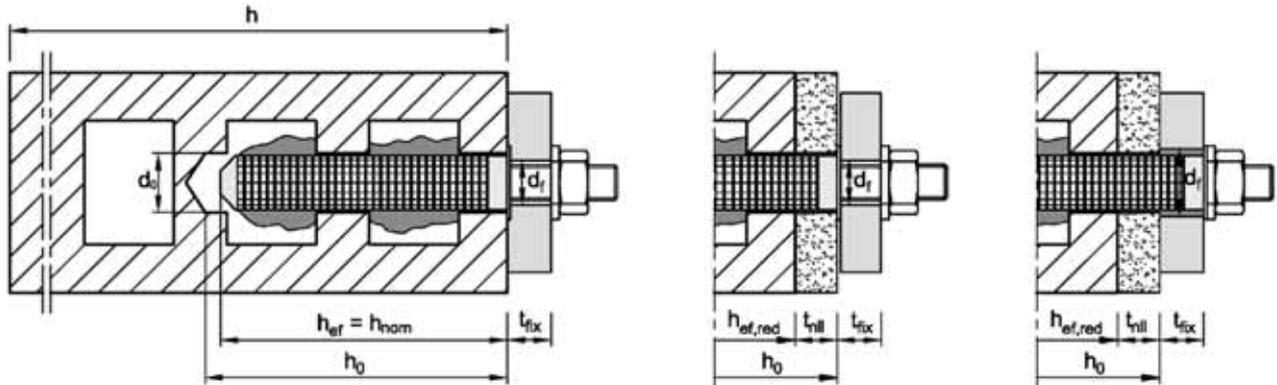
**Installation in hollow brick with or without non-loadbearing layer and/or thermal isolation**
